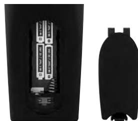
Figure 19 – Remote Battery Compartment
