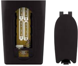
Figure 25 – Remote Battery Compartment
