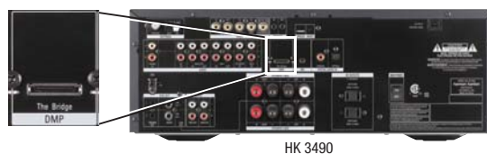
Figure 20 – The Bridge II Connection
