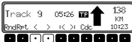
Fast forward / rewind terminates when you release the multifunction key.
