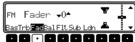
Use the right control knob **⦿** to set the desired fader setting.
