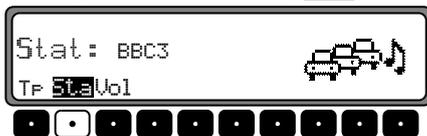
Use the right control knob **⬤** to select the desired TP transmitter. After a short delay without actuation, the selected transmitter is applied.
