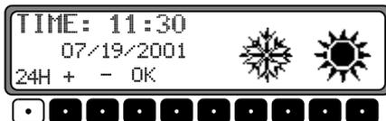
Use the multifunction key **24H** to change the time display from the 24-hour to the 12-hour display.
