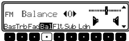
Set the desired balance level using the right control knob **◀▶**.
