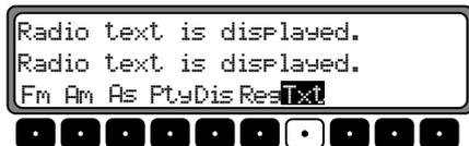
The car radio filters information from the data transmitted by the station and displays as radio text.
