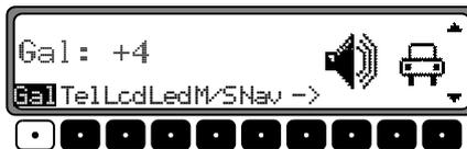
With the GAL settings, the beginning of volume adjustment can be specified according to vehicle speed. The setting is stored automatically.
