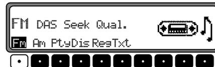
In FM DAS mode, abbreviated names for the receivable stations are displayed above the multifunction keys depending on the settings. In the DAS Seek Qual. mode, stations are arranged in descending signal strength order; in DAS Seek Name mode, they are arranged alphabetically.
