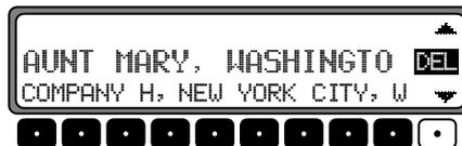
Select the destination to be deleted using the right control knob
