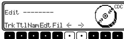
Using the right control knob **⬇**, select the desired letter and press the control to confirm.
