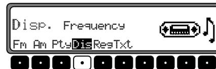
Use multifunction key **Dis** to select Frequency (Frequency display on) or PTY (Frequency display off).
