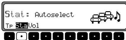
Select **Autoselect** with the right control knob **⬤** and press the control to confirm. After a short delay and without actuation, direct programming is deleted.
