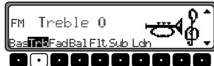
Set the desired treble level using the right control knob **⦿**.
