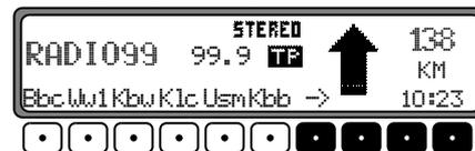
Set the desired station by pressing the key directly below the station designation.
