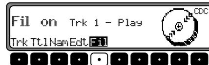
The individual titles of the current CD can be selected using the right control knob **⬇**. It is then possible to select between **Play** (track not filtered) and **Skip** (track filtered out) by pressing the right control knob **⬇**.
