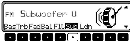
Use the right rotary control **◀▶** to set the desired subwoofer volume level.
