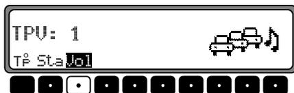
You can select four different settings (0 - 3) with the right control knob
